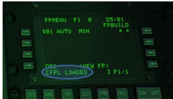
The process is now completed and you can load further WAYPOINTS or FLIGHTPLANS. The last Loading-Process is displayed after sending to CDU in the "Scratchpad" of the Controller.
