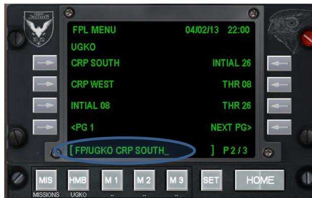
If during the Loading-Process the message [CDU INPUT ERROR ] occurs, the Waypoints are not loaded correctly and the Process must be repeated. You can check this on the WAYPT Page of the CDU. If the count of the Waypoints (at LSK 3R) is not more than before the Loading-Process, there are no Waypoints loaded yet.
